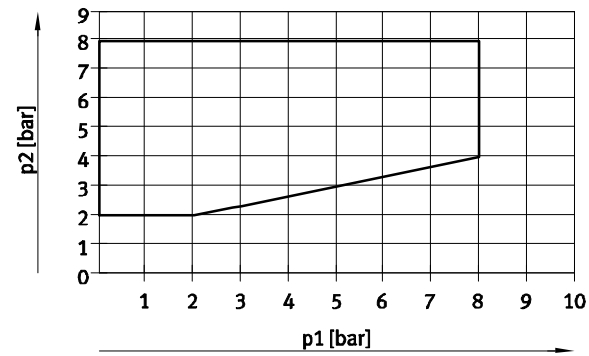
Pilot pressure as a function of operating pressure (operating pressure with external pilot air), pilot pressure 3/2C
