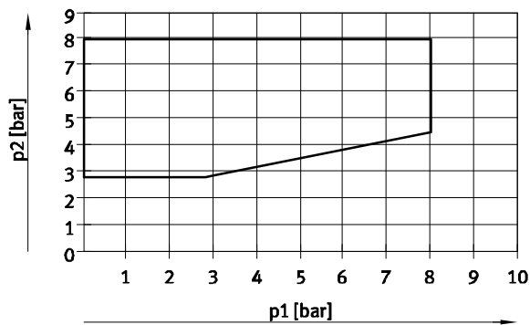
Pilot pressure as a function of operating pressure (operating pressure with external pilot air), pilot pressure 5/2 and 3/2U
